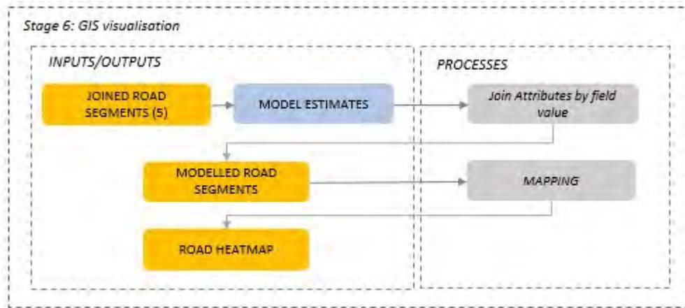
**Figure 73.** Stage 6 joins the processed model outputs and reintegrates them with their corresponding road segments in GIS to produce a heatmap of modelled values.
