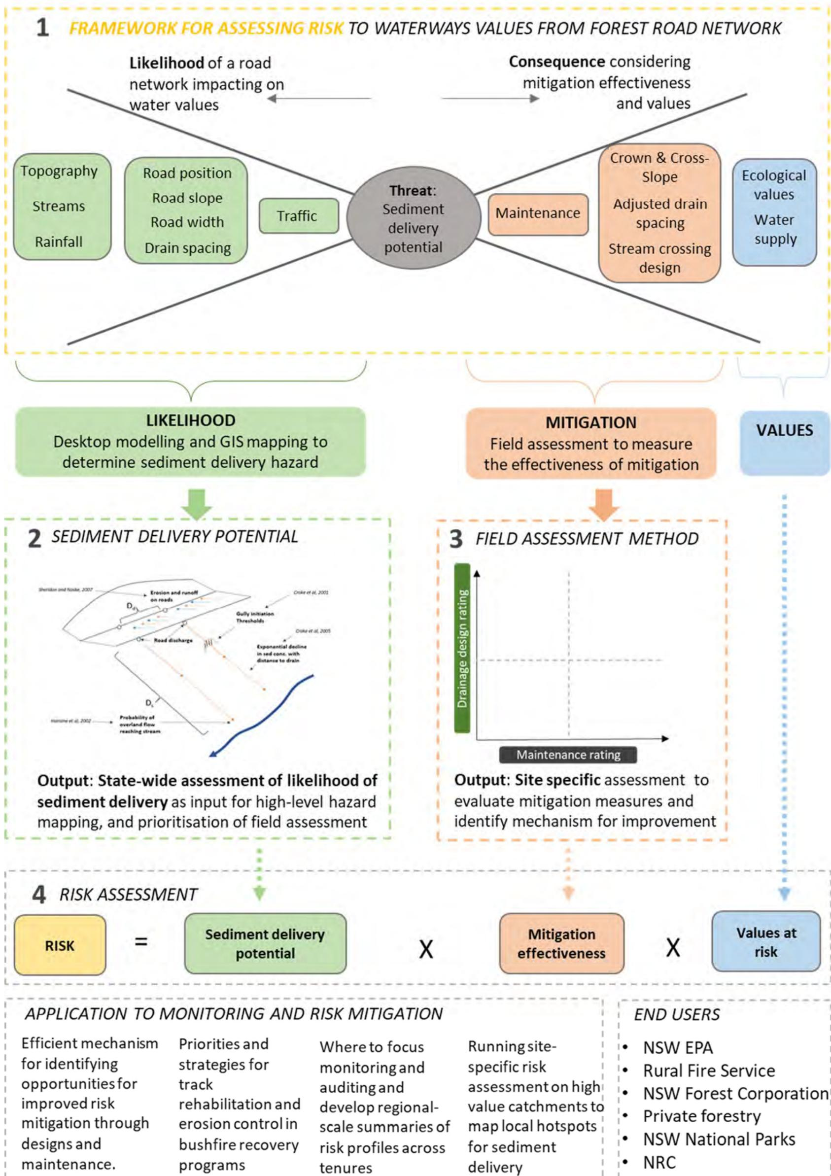
**Figure 1.** Diagram relating the modelling (likelihood) and field assessment (mitigation) components of the program used to calculate the risk forest road networks pose to water quality.
