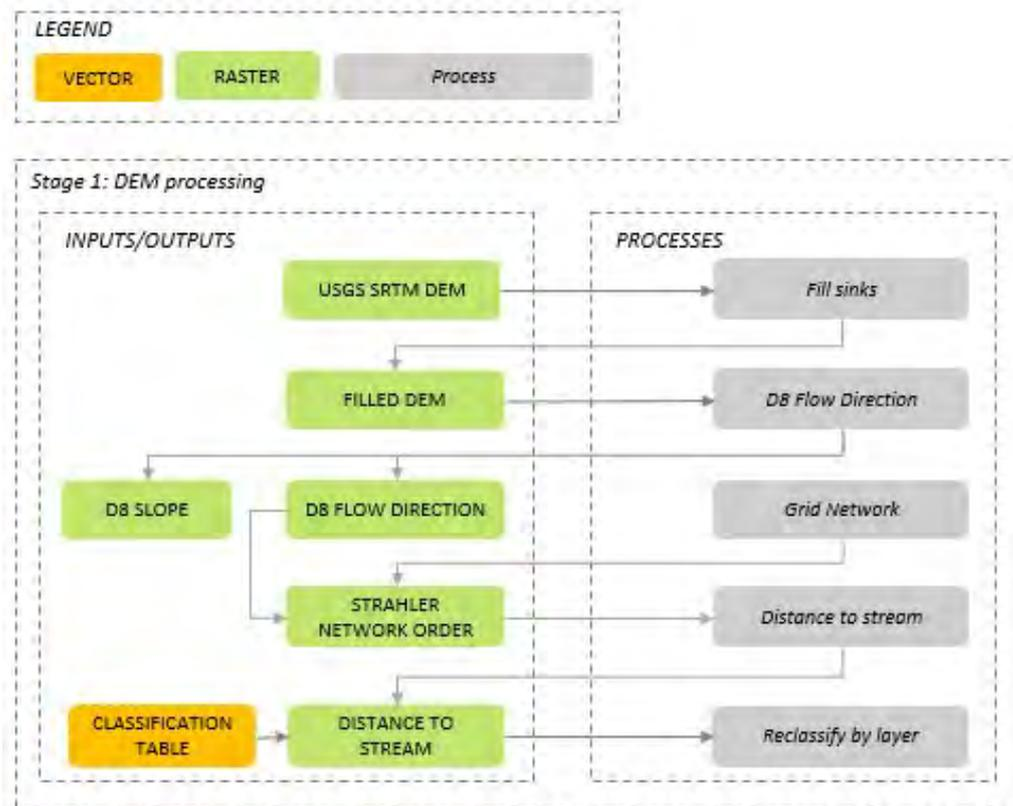
**Figure 68.** Stage 1 outlines the process of conditioning the Digital Elevation Model to calculate distance to streams.
