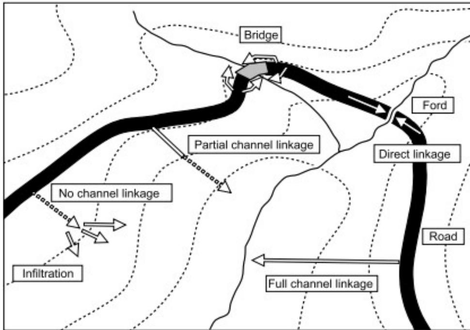
**Figure 40.** The range of potential linkage categories within a forested catchment - from full channel, partial channel, and no channel linkage, to the direct linkage that occurs at a ford or bridge crossing. These categories can be used to determine the degree to which major sources like roads and tracks, are linked to stream (Croke et al, 1999).
