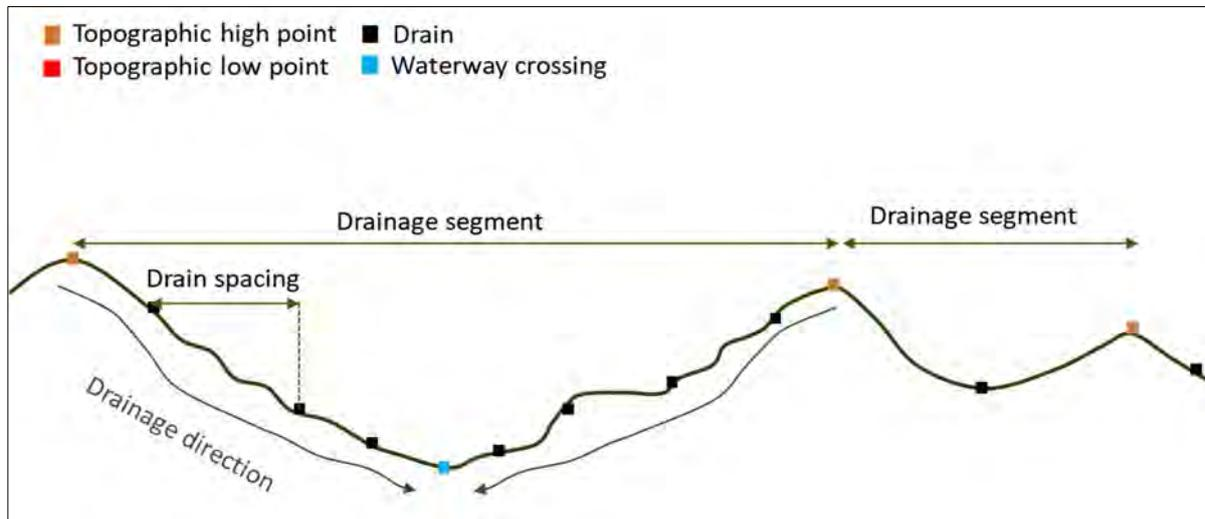
**Figure 21.** A simplified representation of segmenting the drainage network of a road.
