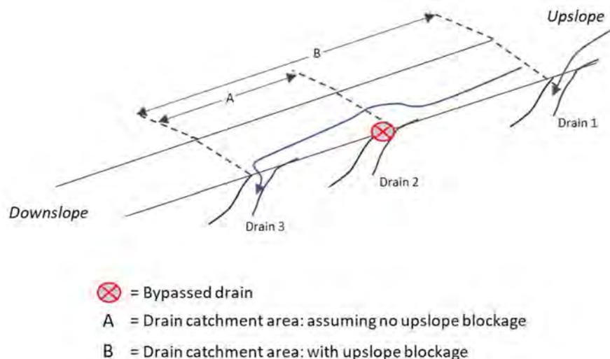
**Figure 22.** Segmenting drain catchment area with and without bypassed drains
