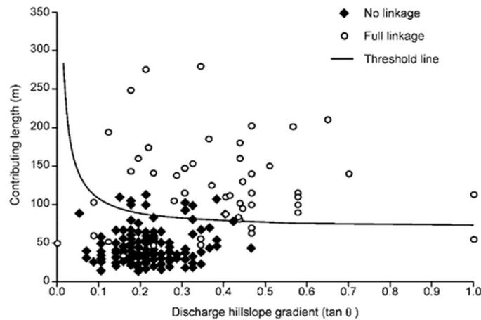
**Figure 43.** Fitted threshold curve separating channelled and non-channelled road drains for the study area (Croke and Mockler 2001).
