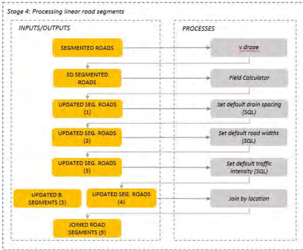
**Figure 71.** Stage 4 takes the segmented road lines and populates their attribute table with key parameters, including those from the buffered road segments, which sampled the raster datasets.
