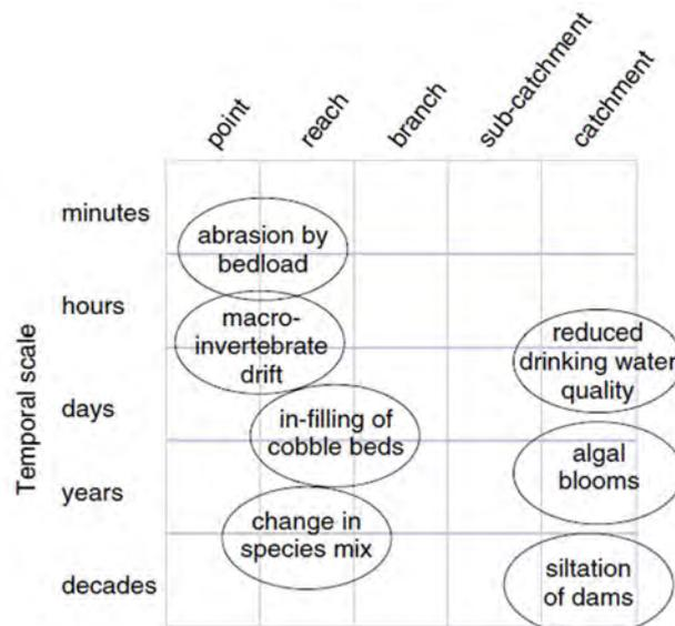
**Figure 34.** The spatial and temporal scale of waterway impacts due to sediment delivery. From Sheridan and Noske (2007)
