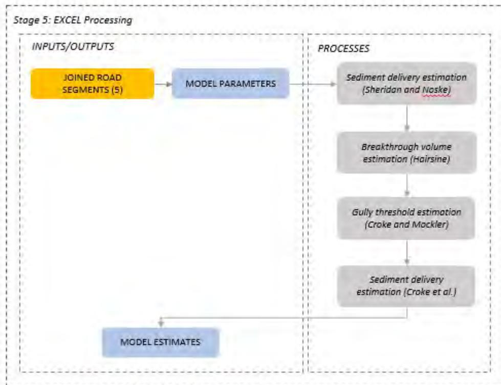
**Figure 72.** Stage 5 takes the attribute data from the parameterised road segments shapefile into Excel to feed the model equations sourced from the literature mentioned.
