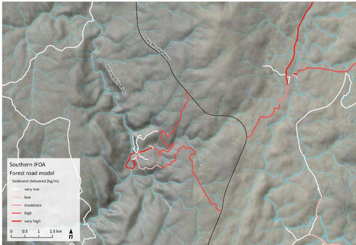
**Figure 50.** Overall sediment delivery hazard in terms of the average sediment delivered by metre of road.
