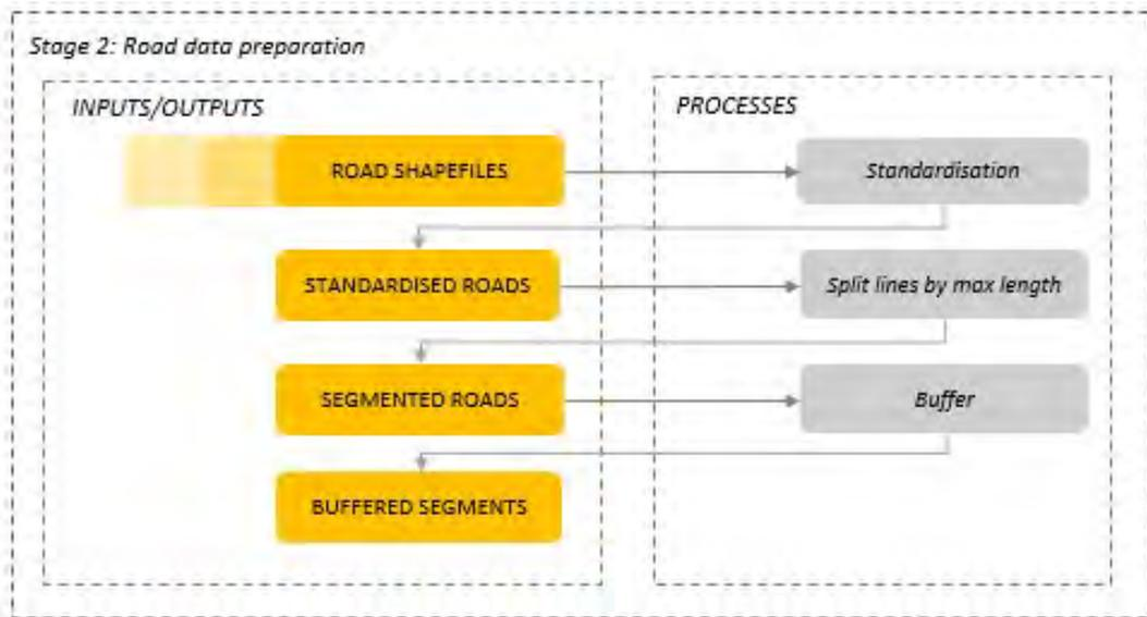
**Figure 69.** Stage 2 prepares the road vector file into segments and buffer zones for subsequent stages.
