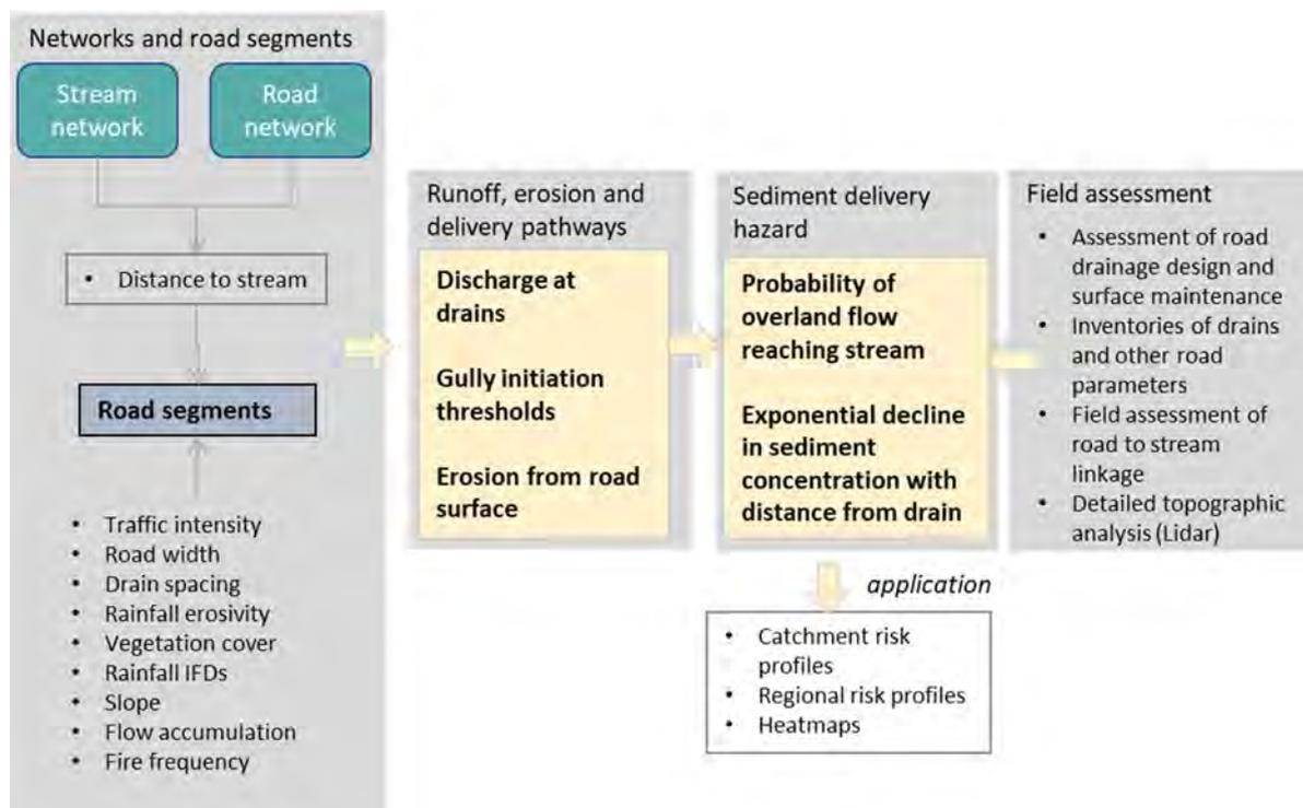
Figure 37. Processing step in implementing the sediment delivery hazard assessment.
