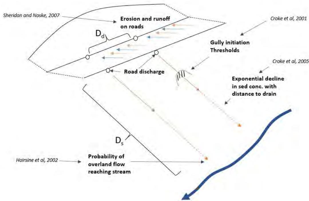
**Figure 41.** How each key process relates to one another in the conceptual model
