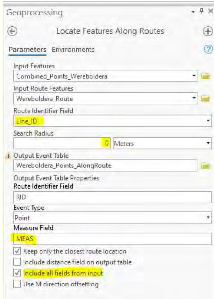
Figure 80. Locate Features Along Routes geoprocessing tool in ArcGIS
