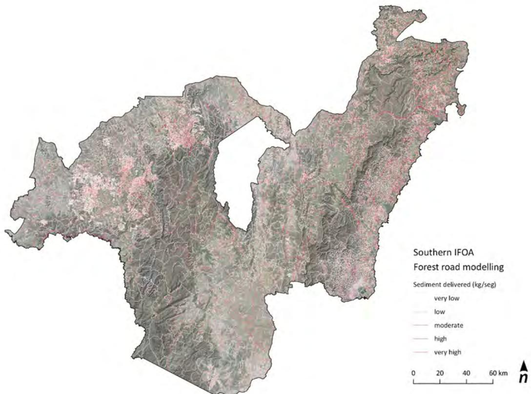
**Figure 47.** Model estimates of sediment delivery hazard by road segment
