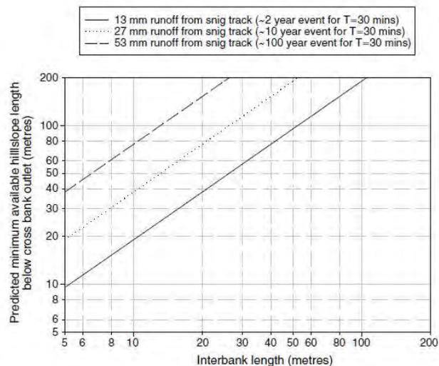
**Figure 44.** An example of how interbank length performs under three different runoff rates. The greater the interbank or outlet spacing, the greater the length of drainage pathway required to avoid delivery to stream.
