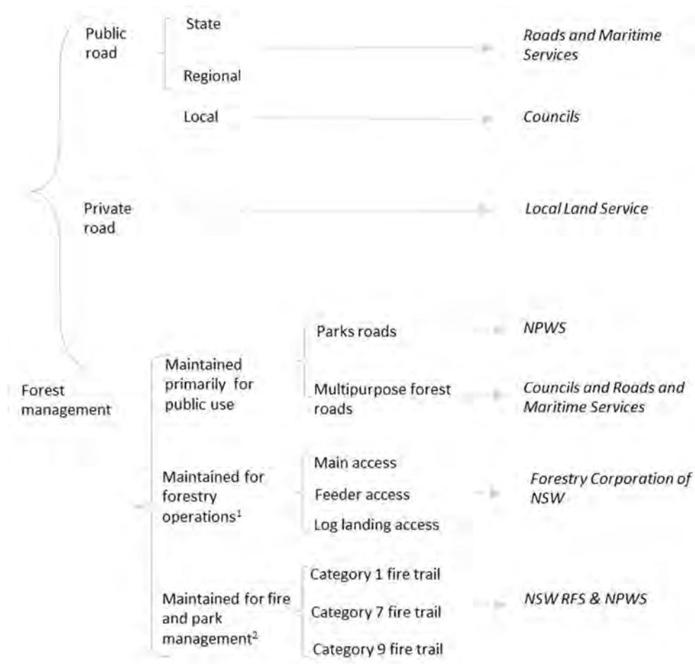
**Figure 30.** Forest road classification for NSW (adapted from Gucinski (2001)). <sup>1</sup>Forestry Roads classification based on Croke and Mockler (2001). <sup>2</sup>Fire trails classification based on Fire Trail Standards (NSW\_RFS, 2019).
