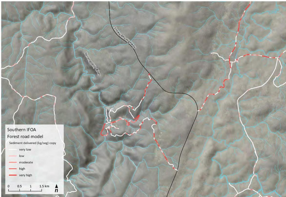
**Figure 49.** Sediment delivery hazard by road segment
