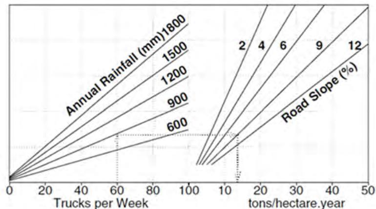
Figure 42. Nomogram for estimating the annual sediment load from gravel surfaced forest roads.
