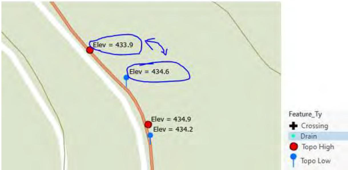
**Figure 84.** Example of False Positive "Topo High" – Field Data collection error
