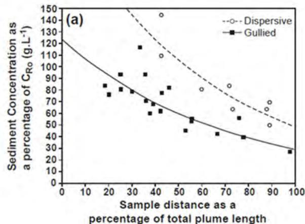
**Figure 45.** The exponential relationship between initial sediment concentration for both dispersive and gullied pathways (Croke et al, 2005).
