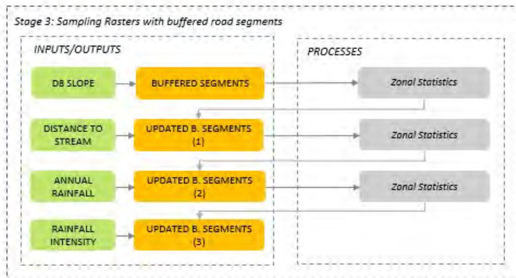
**Figure 70.** Stage 3 utilises the zonal statistics tool to gather the mean values of raster datasets for each buffered road segment.
