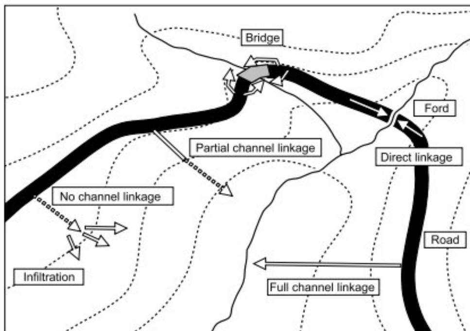
**Figure 36.** The range of potential linkage categories within a forested catchment - from full channel, partial channel, and no channel linkage, to the direct linkage that occurs at a ford or bridge crossing. These categories can be used to determine the degree to which major sources like roads and tracks, are linked to stream (Croke et al, 1999).
