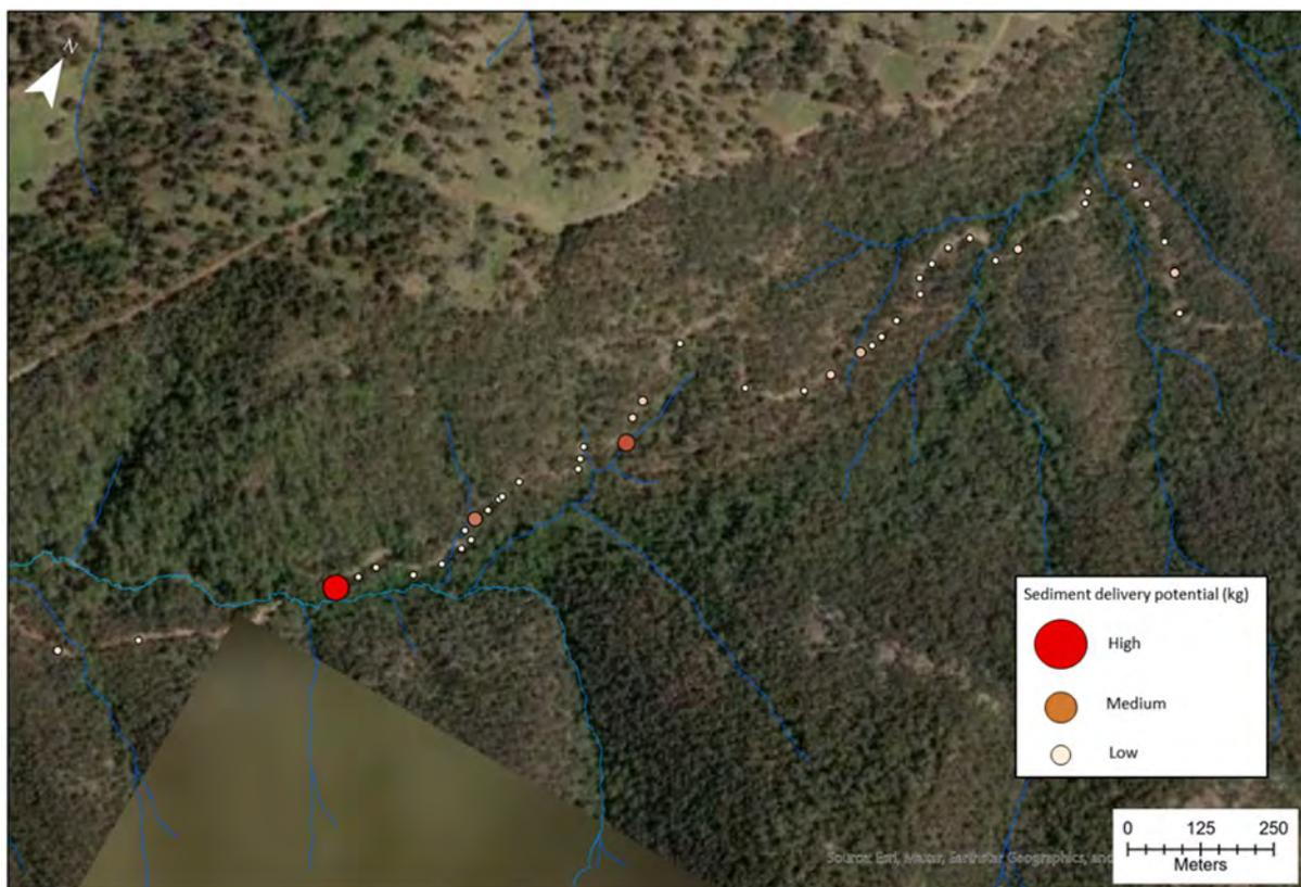
**Figure 26.** Example of the GIS model output, imported to a GIS and symbolised by the base case sediment delivery potential (kg).
